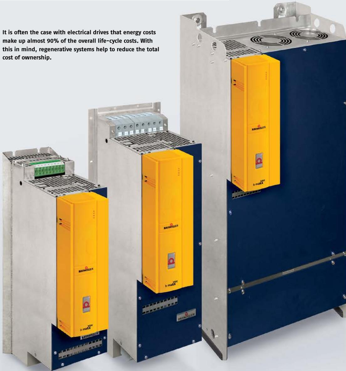
Baumüller's tried-and-tested b maXX automation and drive solution is being expanded with the addition of the new b maXX 4100 series regenerative power supplies. These units work in conjunction with b maXX 4400 series units, and can supply the DC link voltage to one or more drives. By using a b maXX 4100, all excess regenerative brake energy generated by the system is returned to the AC
